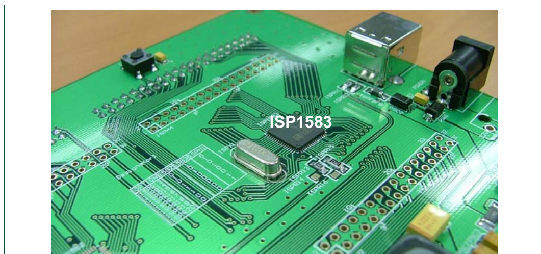
Fig 4. Location of the ISP1583 on the eval board
